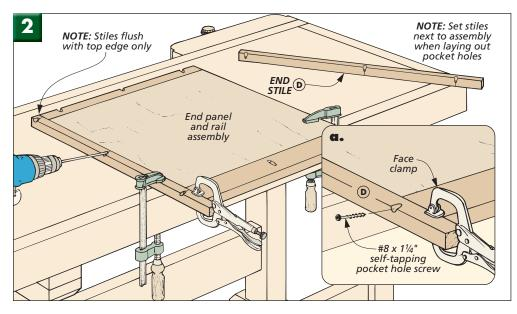
The other thing to note has to do with the use of glue. Technically, the screws should provide plenty of holding power. But to play it safe, it would be a good idea to apply glue too. However, you'll want to use the glue sparingly so you don't have a lot of excess to clean up.
