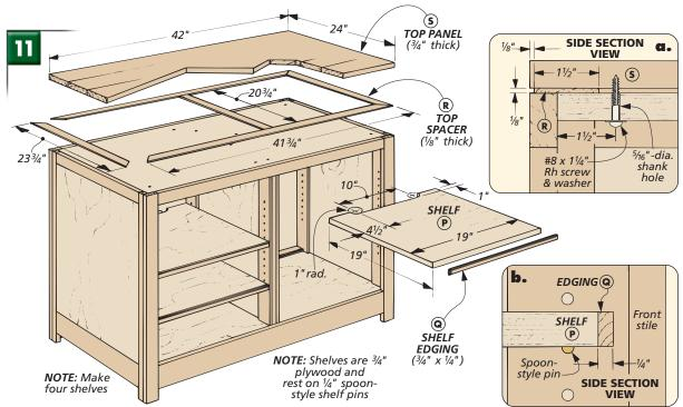
▲ The decorative shadow line on the end assemblies is repeated under the top panel. This time, it's created with thin spacers.
