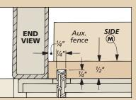
Finally to hold the tongue on the front and back pieces, cut  $\frac{1}{4}$ "  $\times \frac{1}{4}$ " dadoes at the ends of each side piece. (Check the setup with a test piece.)
