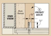
On the front and back pieces, cut a ¼"-wide slot on each end. Raise the blade so the depth matches the thickness of the drawer sides (½").
