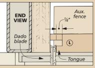
Next create a short tongue on the inside face of each front and back piece. Sneak up on the fence setting until the tongue is ¼" long.
